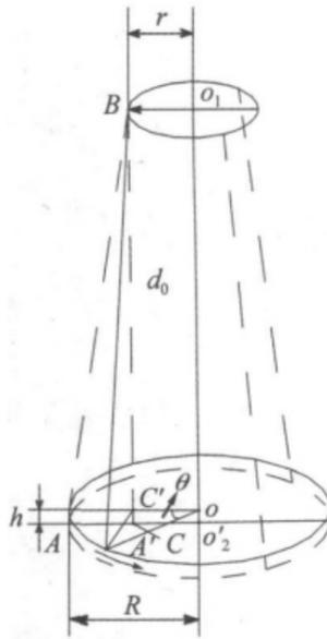
Figure 4: Sketch map of three-wire pendulum <sup>[2]</sup>
