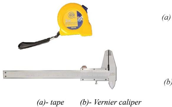
(a)- tape (b)- Vernier caliper
