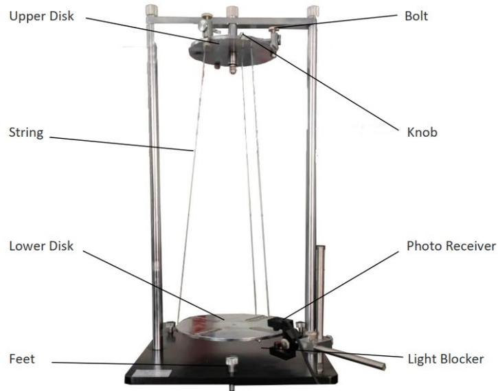
Figure 5: DH4601 The three-string torsional pendulum
