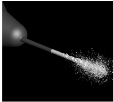
Figure. 7 The volume fraction next to the diesel injector is equal to the surface and Lagrangian particles.
