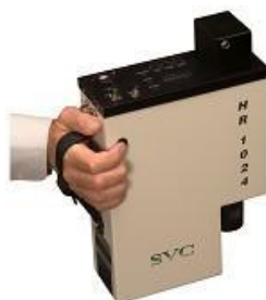
Figure 1. SCVHR 1024i hyperspectral instrument
