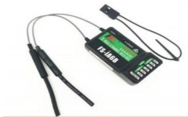
Figure 10: Receiver (receives signals from the remote control)
