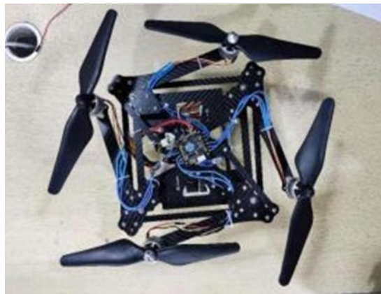
Figure 1: Transformable drone in contracted mode
