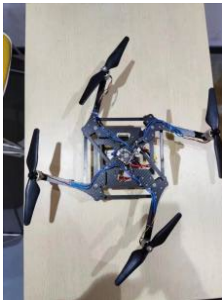
Figure 2: Transformable drone in extended mode
