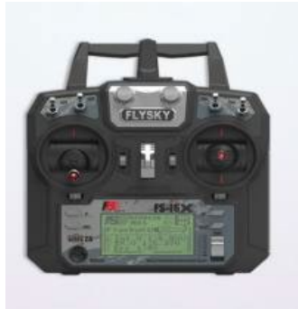
Figure 9: Remote (sends signals to the flight control)
