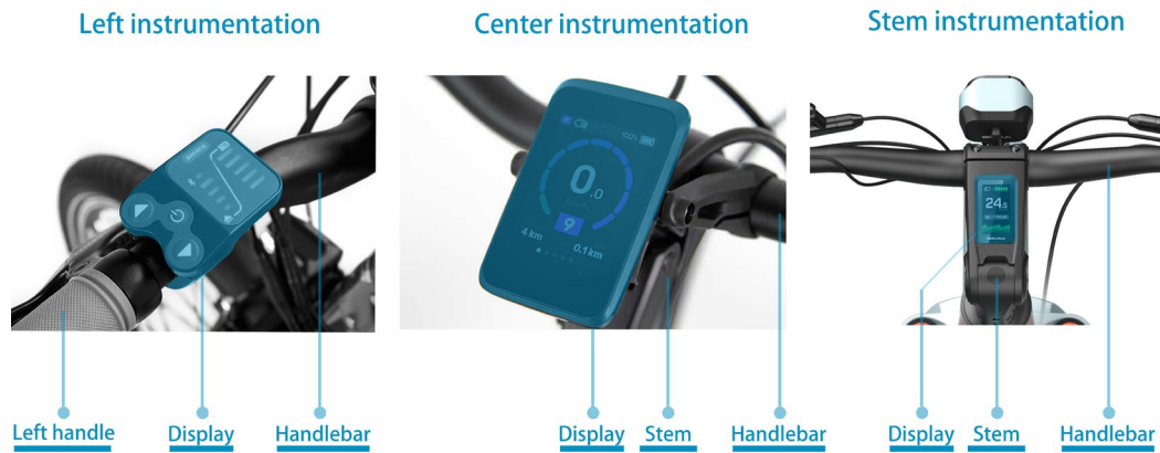
Figure 1: Diagram of pedal-assisted e-bike instrumentation by assembly location (author's own drawing, bicycle image from the Internet)
