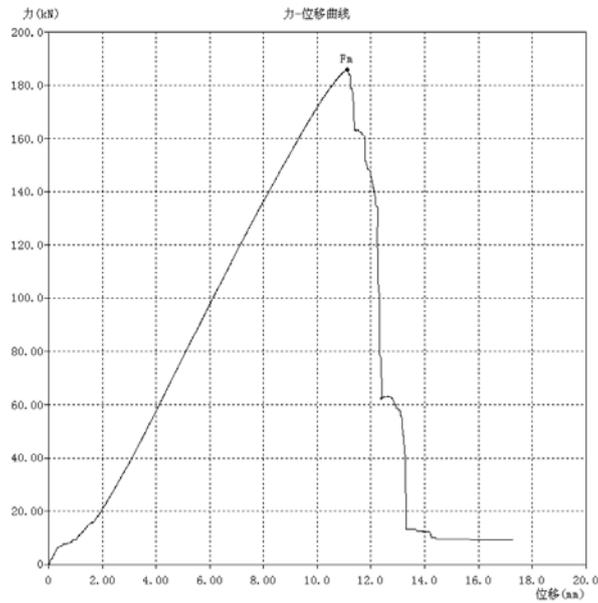
Figure. 3 Load-displacement Curve of Test Specimen S1
