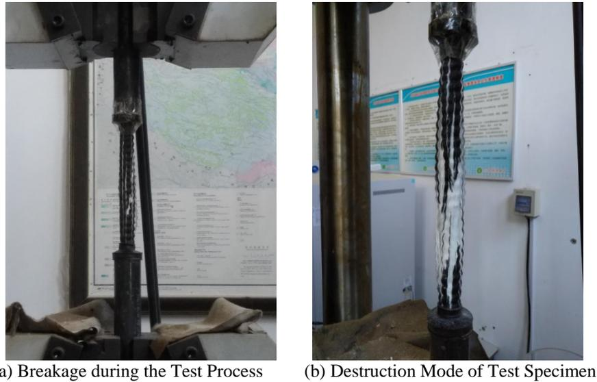
*Figure 2 Breakage of GFRP Test Specimen*
