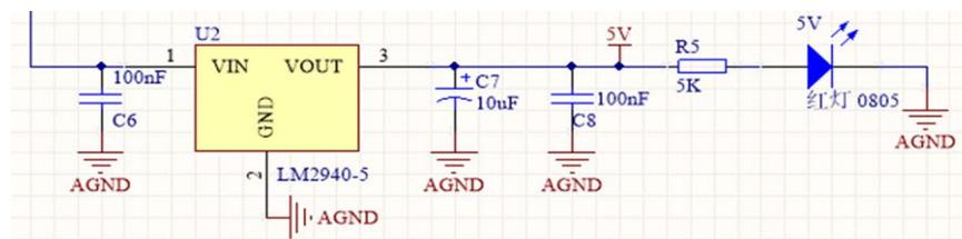
Figure 2. 5V Voltage regulator module Figure.
