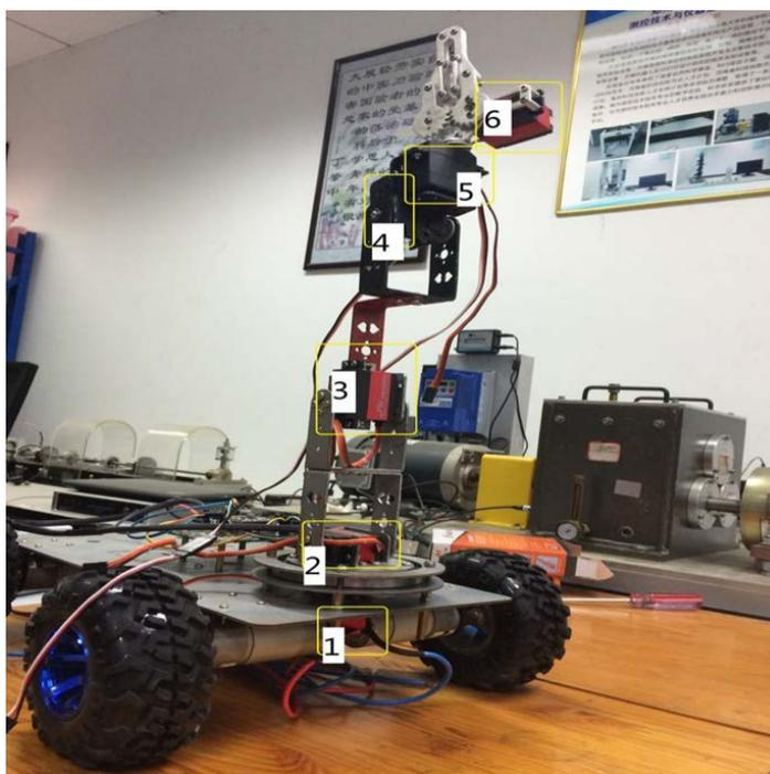
Figure 7. Six steering gear positions in the field weeding mode
