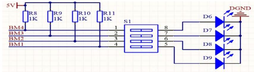
Figure 4. Dial-code switching circuit
