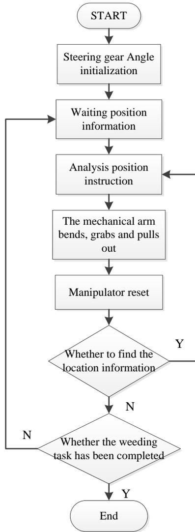
Figure 8. Process flow chart of weeding mode
