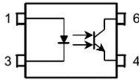
Figure 5. Internal schematic diagram of P181
