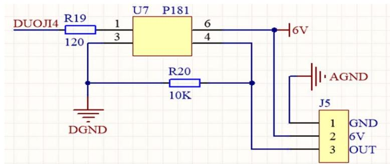
Figure 6. Optocoupler isolation circuit of steering gear in circuit design
