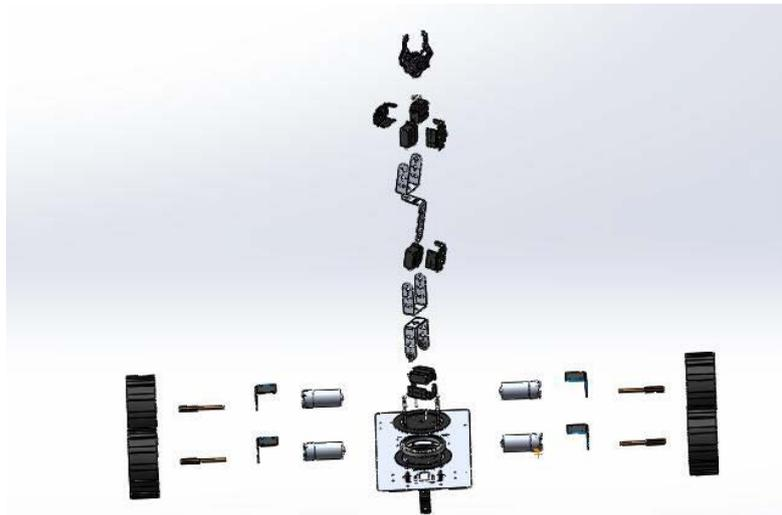
Figure. 1 Explosion view of herbicidal robot.
