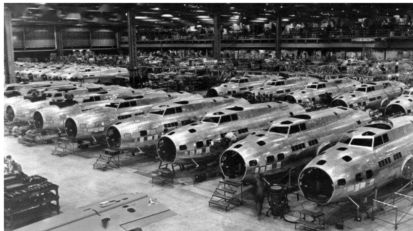
Figure 4. Boeing's large-scale production line for B-17 in 1945, which was the main supply for the US Air Force. [2]
