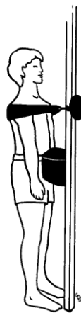
Figure 4 Drawing shows pulling test described by Jorgensen and Nicolaisen. Subject stands facing strain-gauge dynamometer, is then strapped to dynamometer, and attempts maximal backward extension while pelvis is supported. Subject pulls at 60% of MVC under control of supervisor until no longer able to maintain 60% value[5].
