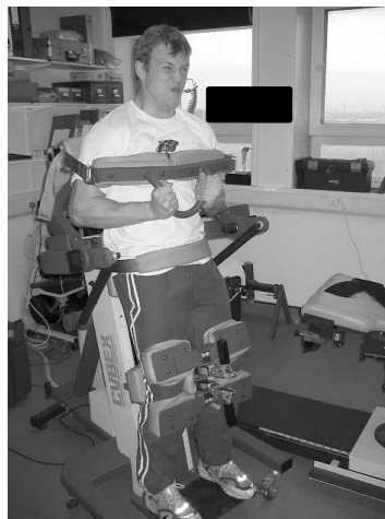
Figure 6 Protocol to test fatigue of the trunk muscles, tests were carried out using the Cybex Norm Isokinetic Dynamometer (Henley Healthcare, Sugarland, Texas, USA) with an incorporated trunk flexion/extension unit[7].
