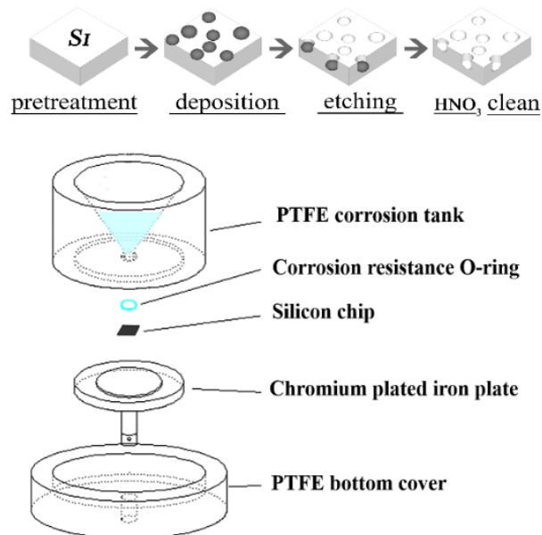
Figure. 1 Schematic illustrations of the whole fabrication process through two-step; Silver Assisted Etching method and the main equipment diagram
