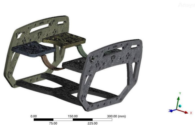
Figure 2: The ROV grid division diagram
