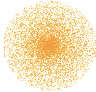
Figure 3: Monte Carlo simulation of the distribution of solar cone energy flow density
