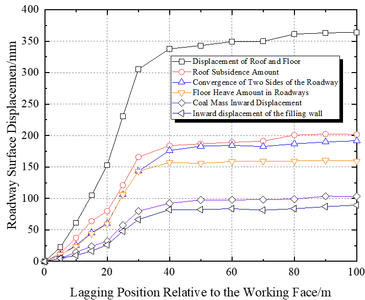
Figure 7 Surface Displacement of the Roadway during the Gob-side Entry Retaining Stage
