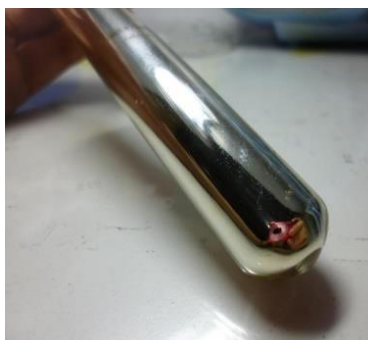
Figure 2: Production of silver mirror
