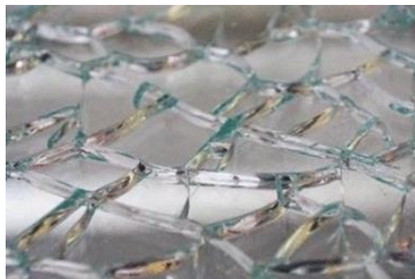
Figure 8: The sample in the low-temperature zone is completely fractured
