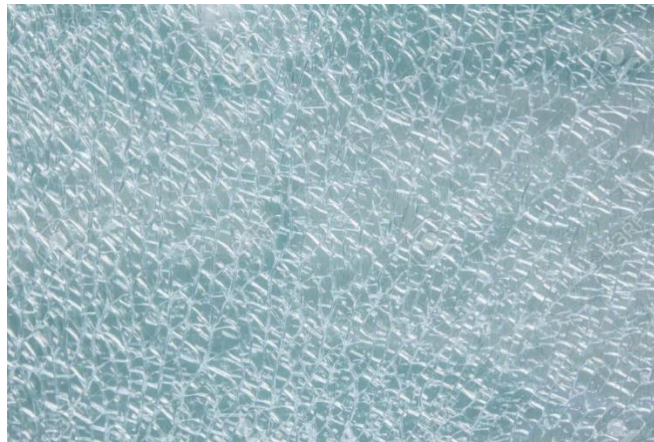
Figure 3: Typical diagram of tempered laminated glass after failure
