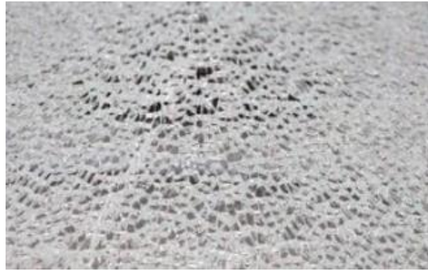
Figure 9: Fracture lines of samples in a high-temperature area
