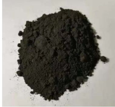
Figure. 3 Containing Converter Sludge
