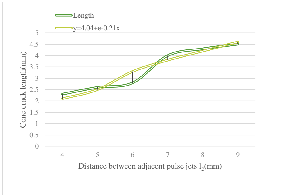
Figure 2: The length of cone cracks in the rock under different jet column spacing
