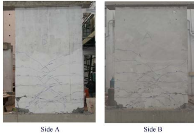
Figure 12. The overall diagram of the YZ12 test piece
