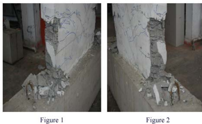
Figure 11. Concrete in the compression zone at the later stage of YZ16
