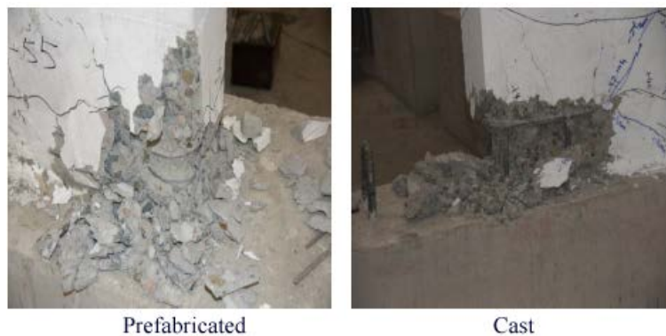
Figure 19. The destruction phenomenon in the compression zone of shear wall
