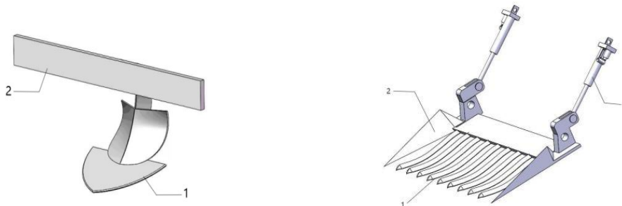
Figure 2: Soil plowing mechanism 1-plough shovel 2-irons (Left)
