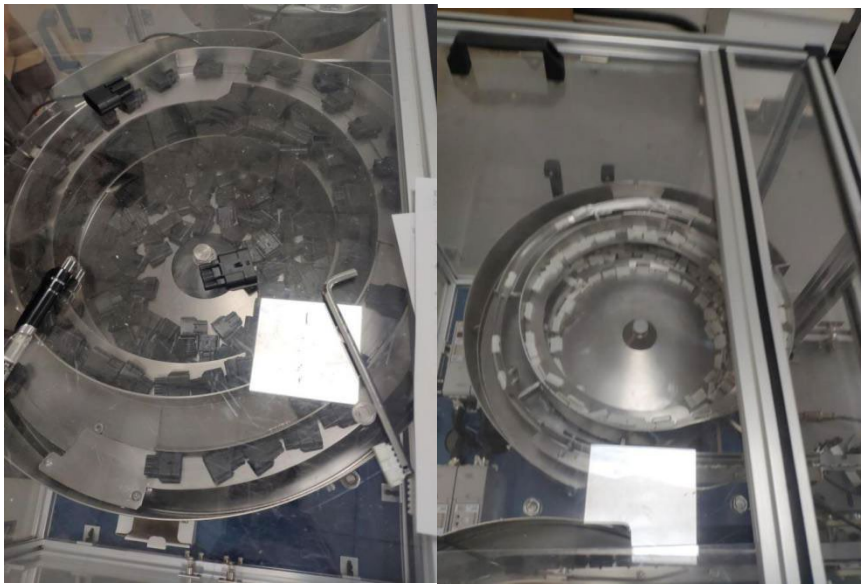
Figure 1: Vibrating plate material supply
