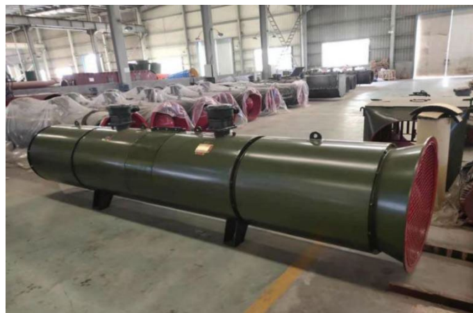
Fig. 1 FBDNo7.0/2×45 contra-rotating axial-flow fan for mining
