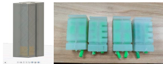
Figure 2 3D model of the first version of the silicone mold and Silicone airbags cooled and removed from external supports
