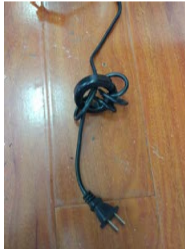
Figure 7 Winding the magnetic ring on the power cord
