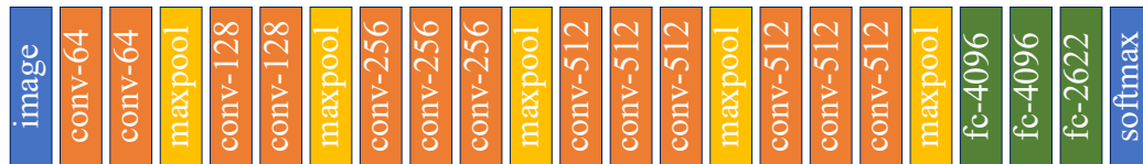
Figure 2: Structure of the VGGFace model.
