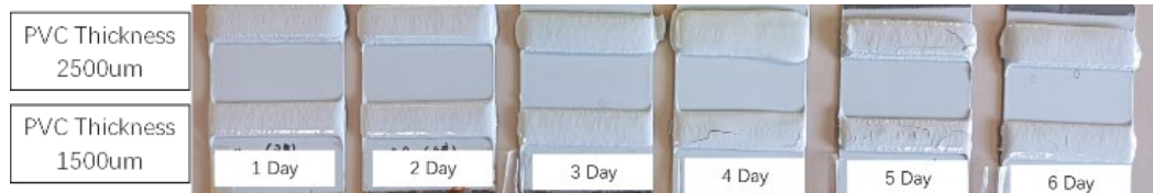
Figure 2: Crack status of different PVC thickness
