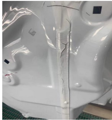
Figure 1: Crack status of paint on PVC surface
