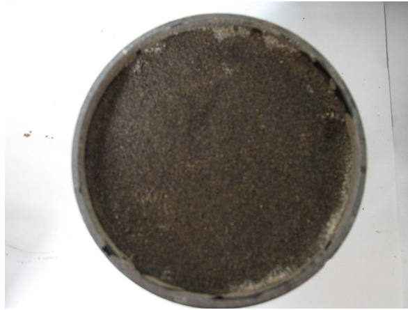
Figure 2. Lighter-colored samples after emulsion penetration
