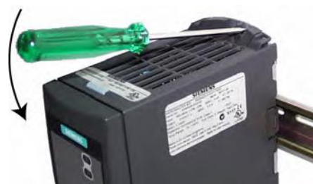
Figure 2: Mounting the inverter onto a 35 mm standard rail (EN 50022)
